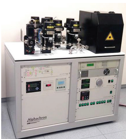
The Alphachron™ automated helium thermochronology instrument is a turnkey system for the automated extraction and measurement of radiogenic helium from mineral samples
