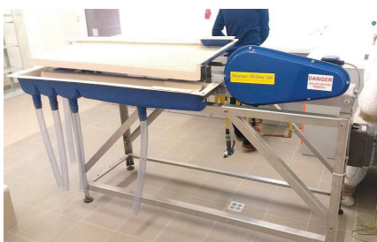
Wilfley shaking table is used for gravity mineral separation from suspension
