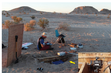
Displacement monitoring on the Superstition Hills Fault, California, using a TM71 mechanical dilatometer with automated data recording
